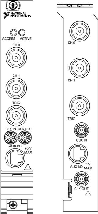
**Table 1.** PXI/PCI-5124 Front Panel Connectors
