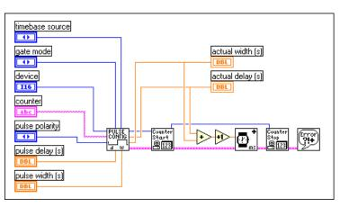
Figure 24-7. Diagram of Delayed Pulse-Int (DAQ-STC) VI
