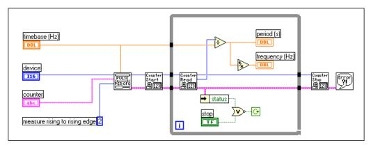
Figure 26-11. Measuring Period Using Intermediate Counter VIs
