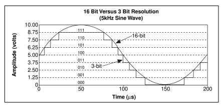
Figure 5-4. The Effects of Resolution on ADC Precision
