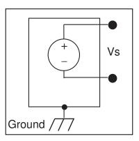
Figure 5-3. Floating Signal Sources
