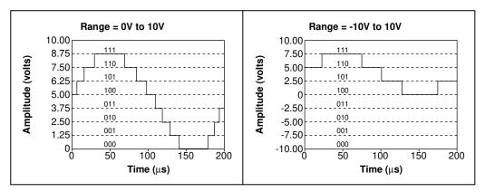
Figure 5-5. The Effects of Range on ADC Precision
