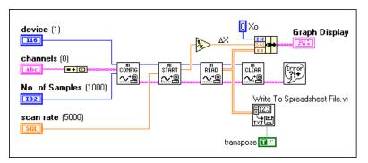
Figure 7-8. Writing to a Spreadsheet File after Acquisition
