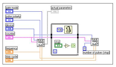
Figure 24-13. Diagram of Cont Pulse Train-Easy (DAQ-STC) VI
