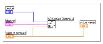
Figure 11-2. Single Immediate Update Using the AO Update Channel VI
