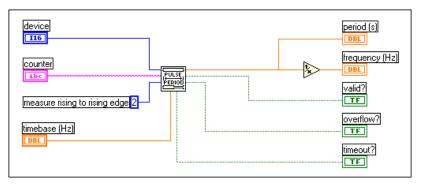
Figure 26-9. Diagram of Measure Period-Easy (DAQ-STC) VI
