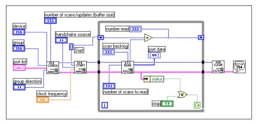
Figure 17-9. Digital Handshaking Using a Circular Buffer
