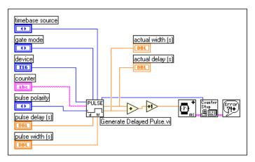
Figure 24-6. Diagram of Delayed Pulse-Easy (DAQ-STC) VI
