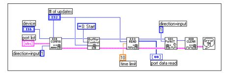
Figure 17-8. Reading Data with the Digital VIs Using Digital Handshaking
