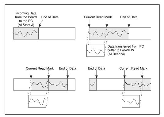
Figure 7-9. How a Circular Buffer Works
