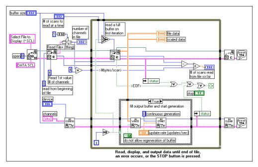
Figure 12-6. Display and Output Acq'd File (Scaled) VI
