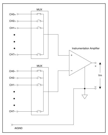
Figure 5-7. 8-Channel Differential Measurement System
