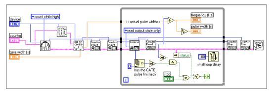
Figure 26-7. Frequency Measurement Example Using Intermediate VIs
