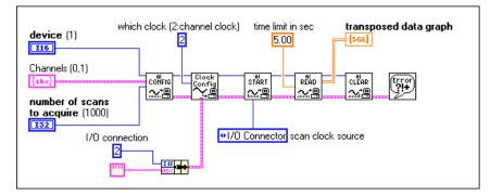
Figure 9-7. Controlling the Scan and Channel Clock Simultaneously
