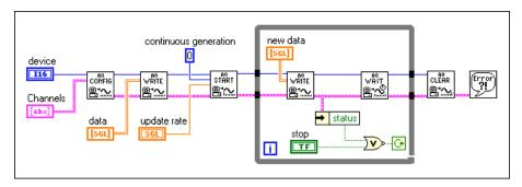
Figure 12-5. Circular Buffered Waveform Generation Using Intermediate VIs
