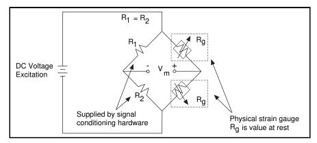
Figure 21-7. Half-Bridge Strain Gauge
