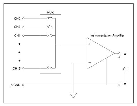
Figure 5-9. 16-Channel RSE Measurement System
