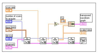
Figure 7-4. Using the Intermediate VIs to Acquire Multiple Waveforms
