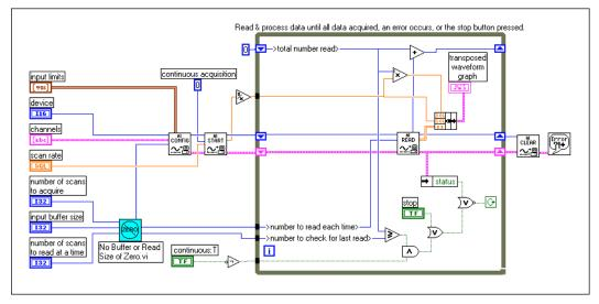
Figure 7-10. Continuously Acquiring Data with the Intermediate VIs
