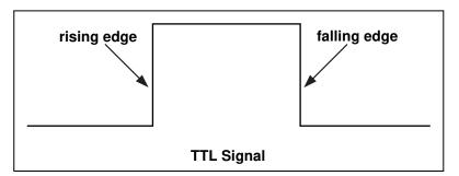
Figure 9-3. Example of a TTL Signal
