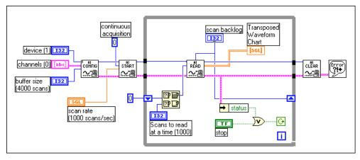
Figure 7-12. Basic Circular-Buffered Analog Input Using the Intermediate VIs
