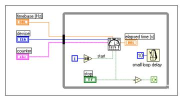
Figure 27-10. Diagram of Count Time-Easy (DAQ-STC) VI
