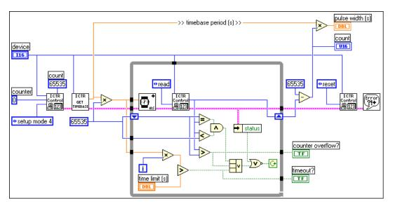
Figure 25-7. Diagram of Measure Short Pulse Width (8253) VI
