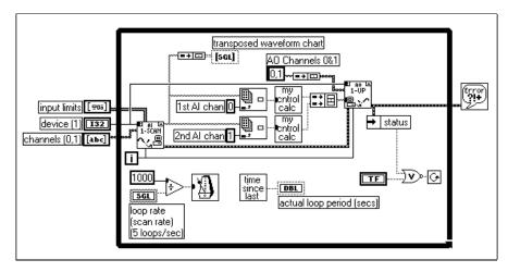
The following diagram shows how to perform software-timed analog I/O using the AI Read One Scan and AO Write One Update VIs.
