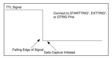
Figure 8-1. Diagram of a Digital Trigger
