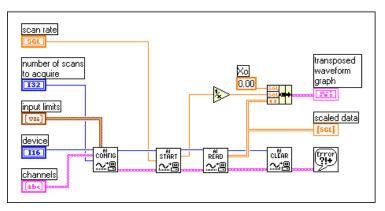
Figure 7-6. Simple Buffered Analog Input with Graphing
