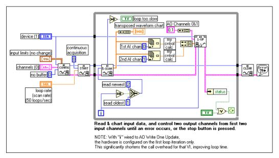
Figure 6-8. Analog IO Control Loop (HW-Timed) VI Block Diagram
