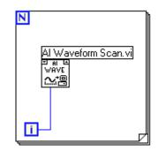
Wiring the **iteration** input this way means the device is only configured on the first I/O operation. Subsequent I/O operations use the existing configuration.
