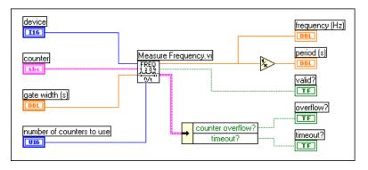
Figure 26-6. Diagram of Measure Frequency-Easy (9513) VI
