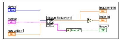
Figure 26-5. Diagram of Measure Frequency-Easy (DAQ-STC) VI
