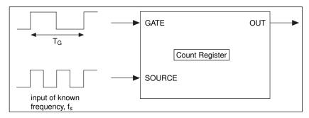
Figure 26-2. Measuring a Square Wave Period
