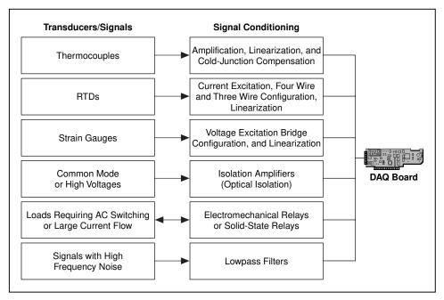
Figure 18-1. Common Types of Transducers/Signals and Signal Conditioning
