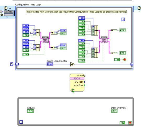
11. Place a Write Accessor node in the While Loop to the right of the **Acquire** control.
