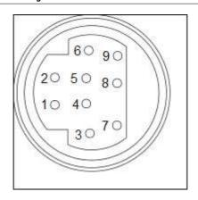
Table 4. DIO 9-Pin DIN Connector Pinout
