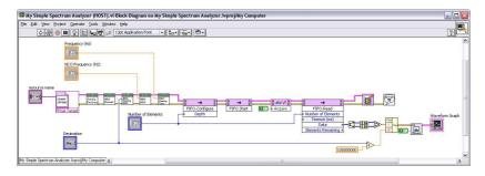
Divide the decimation rate value by 100M, which is the default Sample Clock rate of the ADCs, and wire the output to the dt input of the Build Waveform VI.
