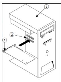
Figure 1. Module Installation
