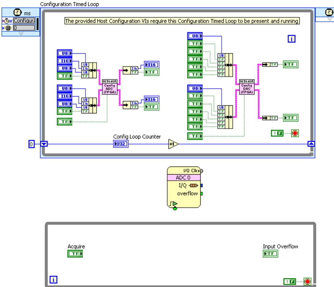
11. Place a Write Accessor node in the While Loop to the right of the **Acquire** control.
