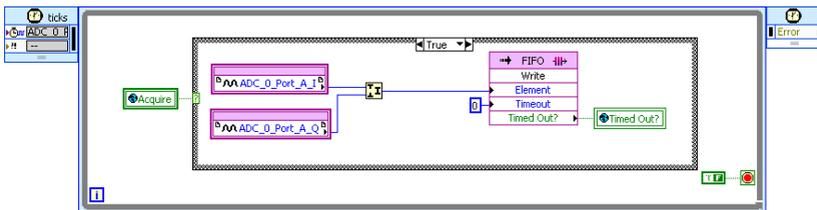
The acquired I and Q data, which are 16-bit values, are packed into a 32-bit value by the Join Numbers function. The packed value is then sent to the FIFO, which transfers the data to the host computer using DMA.
