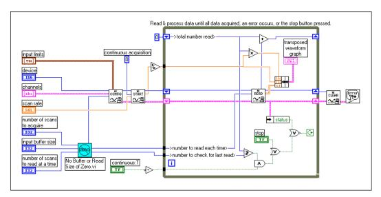
Figure 7-10. Continuously Acquiring Data with the Intermediate VIs
