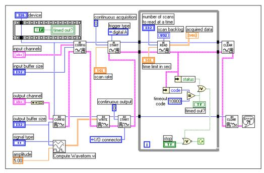
Figure 14-4. Simultaneous Input/Output Using the Simul Al/AO Buffered Trigger (Legacy MIO) VI
