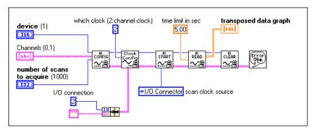
Figure 9-7. Controlling the Scan and Channel Clock Simultaneously
