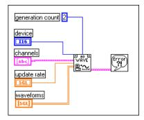
Figure 12-2. Waveform Generation Using the AO Waveform Gen VI
