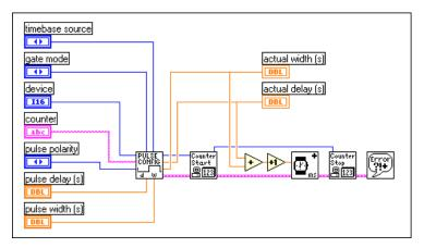
Figure 24-7. Diagram of Delayed Pulse-Int (DAQ-STC) VI
