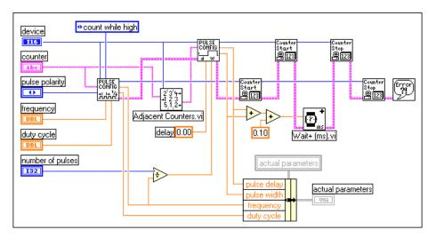
Figure 24-19. Diagram of Finite Pulse Train-Int (DAQ-STC) VI
