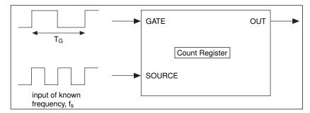
Figure 26-2. Measuring a Square Wave Period
