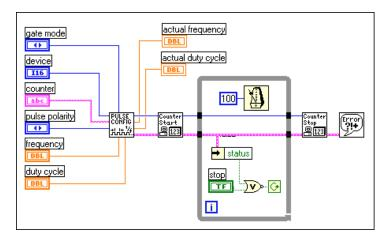
Figure 24-14. Diagram of Cont Pulse Train-Int (DAQ-STC) VI
