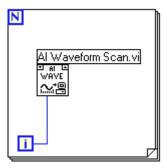
Wiring the **iteration** input this way means the device is only configured on the first I/O operation. Subsequent I/O operations use the existing configuration.
