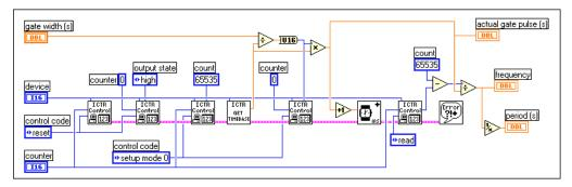
Figure 26-8. Diagram of Measure Frequency > 1 kHz (8253) VI
