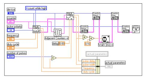
Figure 24-19. Diagram of Finite Pulse Train-Int (DAQ-STC) VI
