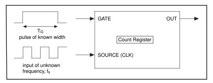
Figure 26-1. Measuring Square Wave Frequency
