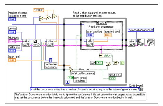
Figure 7-11. Continuous Acq&Chart (Async Occurrence) VI
