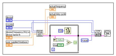
Figure 24-16. Diagram of Cont Pulse Train (8253) VI
