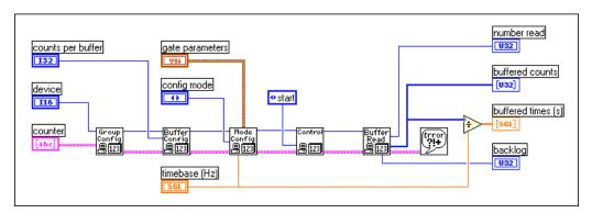
Figure 25-9. Diagram of Meas Buffered Pulse-Period (DAQ-STC).vi
