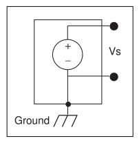
Figure 5-2. Grounded Signal Sources
