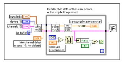
Figure 6-6. The Cont Acq&Chart (Immediate) VI Block Diagram
