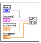
Figure 12-1. Waveform Generation Using the AO Generate Waveforms VI
