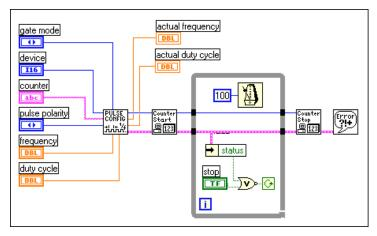
Figure 24-14. Diagram of Cont Pulse Train-Int (DAQ-STC) VI
