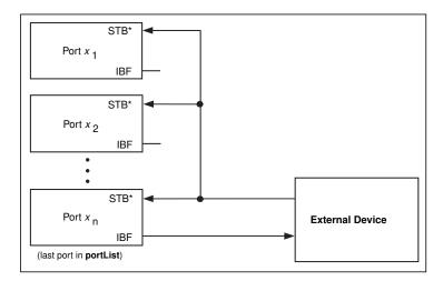
Figure 17-1. Connecting Signal Lines for Digital Input
