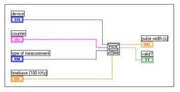
Figure 25-5. Diagram of Measure Pulse Width (9513) VI
