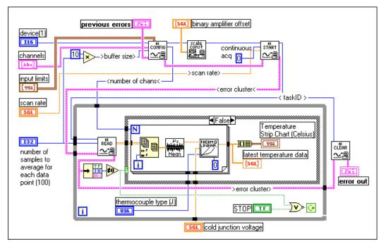
Figure 21-4. Continuously Acquiring Data Using Intermediate VIs
