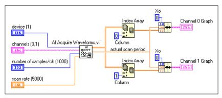
Figure 7-5. Simple Buffered Analog Input Example
