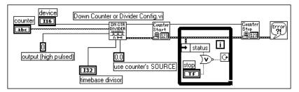
Figure 28-2. Programming a Single Divider for Frequency Division
