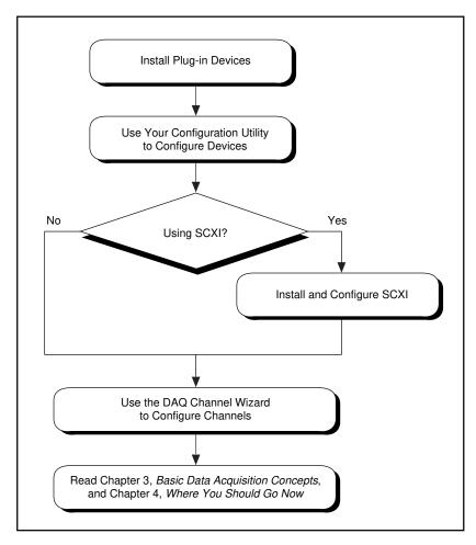
Figure 2-1. Installing and Configuring DAQ Devices
