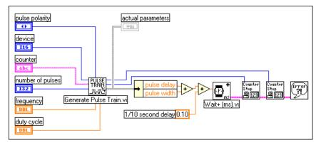
Figure 24-18. Diagram of Finite Pulse Train-Easy (DAQ-STC) VI
