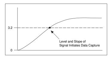
Figure 8-4. Diagram of an Analog Trigger
