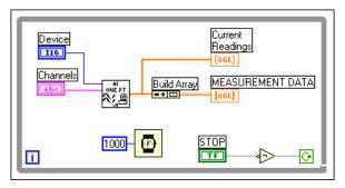
Figure 21-1. Continuous Transducer Measurement VI
