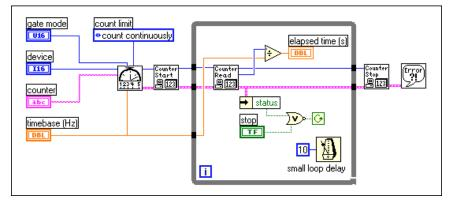
Figure 27-11. Diagram of Count Time-Int (DAQ-STC) VI
