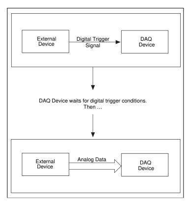
Figure 8-2. Digital Triggering with Your DAQ Device
