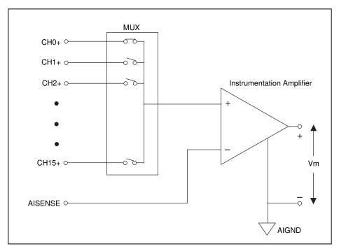
Figure 5-10. 16-Channel NRSE Measurement System
