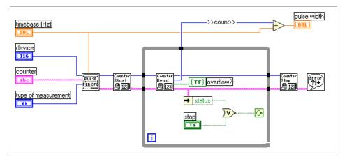
Figure 25-8. Measuring Pulse Width with Intermediate VIs
