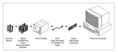
Figure 19-2. Components of an SCXI System
