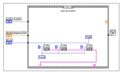
Figure 24-23. Frame 0 of Finite Pulse Train (8253) VI
