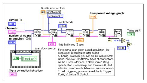
Figure 9-6. Externally Controlling Your Scan Clock with the Getting Started Analog Input Example VI
