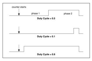
Figure 24-1. Pulse Duty Cycles
