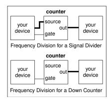
Figure 28-1. Wiring Your Counters for Frequency Division
