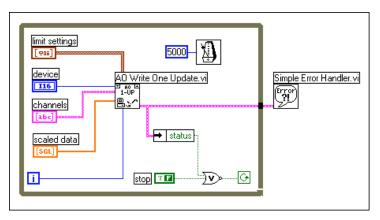
Figure 11-4. Multiple Immediate Updates Using Intermediate VI
