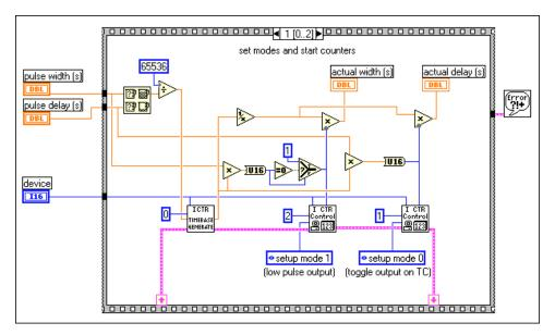
Figure 24-10. Frame 1 of Delayed Pulse (8253) VI
