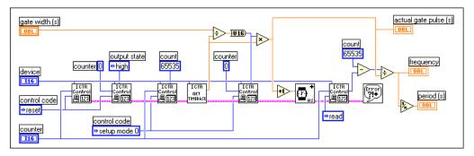
Figure 26-8 shows the Measure Frequency > 1kHz (8253) VI located in labview\examples\daq\8253.11b.
