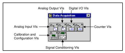
Figure 3-2. Data Acquisition VIs Palette
