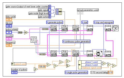
Figure 24-21. Diagram of Finite Pulse Train-Adv (DAQ-STC) VI
