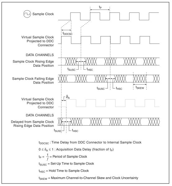
Figure 3. Acquisition Timing Diagram
