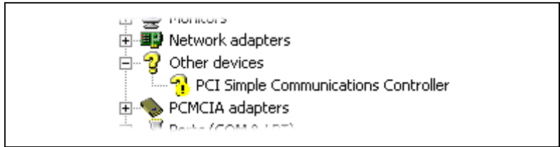
Figure C-2. CAN Interface That has Not Been Recognized Properly
