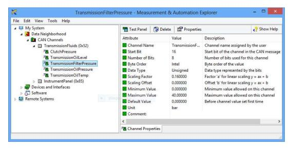
Figure 2-2. CAN Channels in MAX
