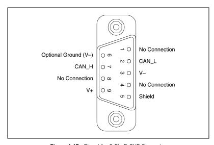
Figure 4-17. Pinout for 9-Pin D-SUB Connector
