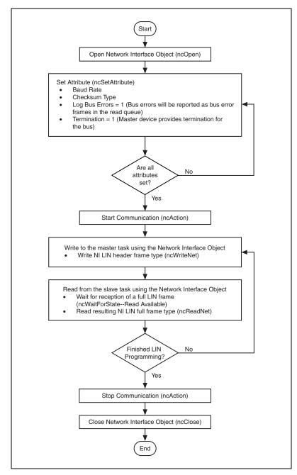
**Figure 9-6.** Frame API – LIN interface provides simple access to a single slave device that publishes data
