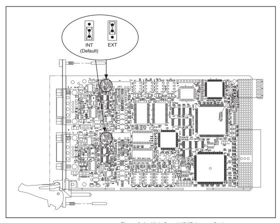
Figure 3-4. High-Speed VBAT Jumper Settings
