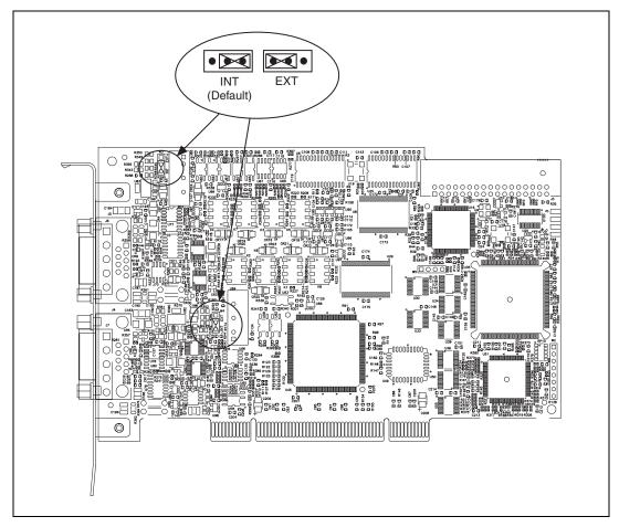
Figure 3-2. Low-Speed/Fault-Tolerant VBAT Jumper Settings
