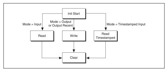
Figure 6-2. Basic Programming Model for Channel API
