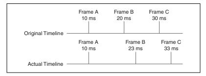
Figure 11-13. Example with Time Recovery Disabled
