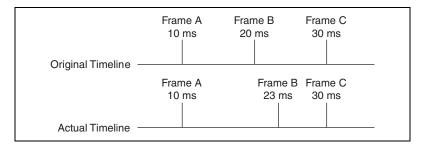
Figure 10-10. Example with Time Recovery Enabled
