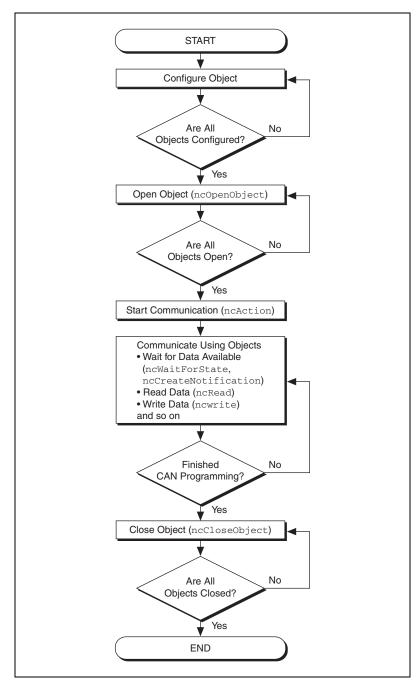
Figure 9-1. Programming Model for NI-CAN Frame API
