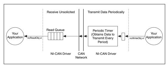
Figure 10-1. Example of Periodic Transmission
