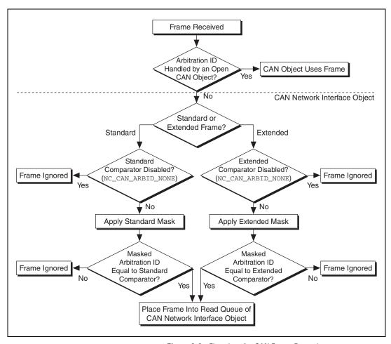
Figure 9-8. Flowchart for CAN Frame Reception
