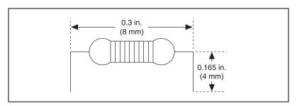
Figure 4-11. Preparing Lead Wires of Replacement Resistors
