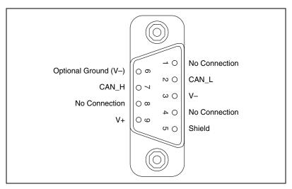
Figure 4-14. Pinout for 9-Pin D-SUB Connector
