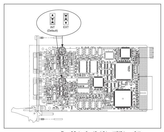
Figure 3-5. Low-Speed/Fault-Tolerant VBAT Jumper Settings
