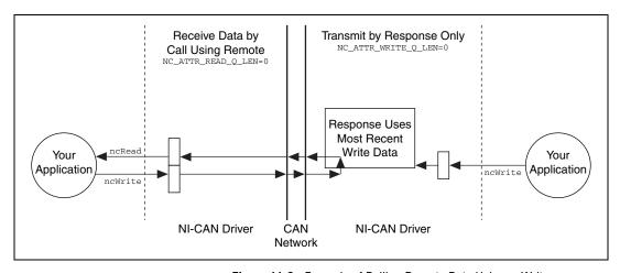
**Figure 11-6.** Example of Polling Remote Data Using ncWrite
