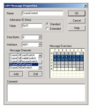
Figure 1-8. Example of CruiseControl Message
