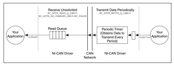
Figure 11-5. Example of Periodic Transmission
