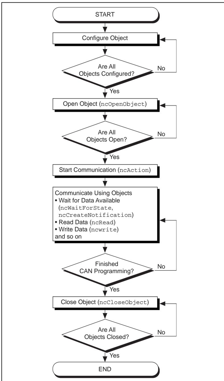
**Figure 2-1.** General Program Steps Using NI-CAN Functions
