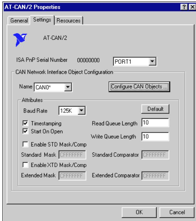
**Figure 5-1.** NI-CAN Settings Dialog Box for an AT-CAN/2
