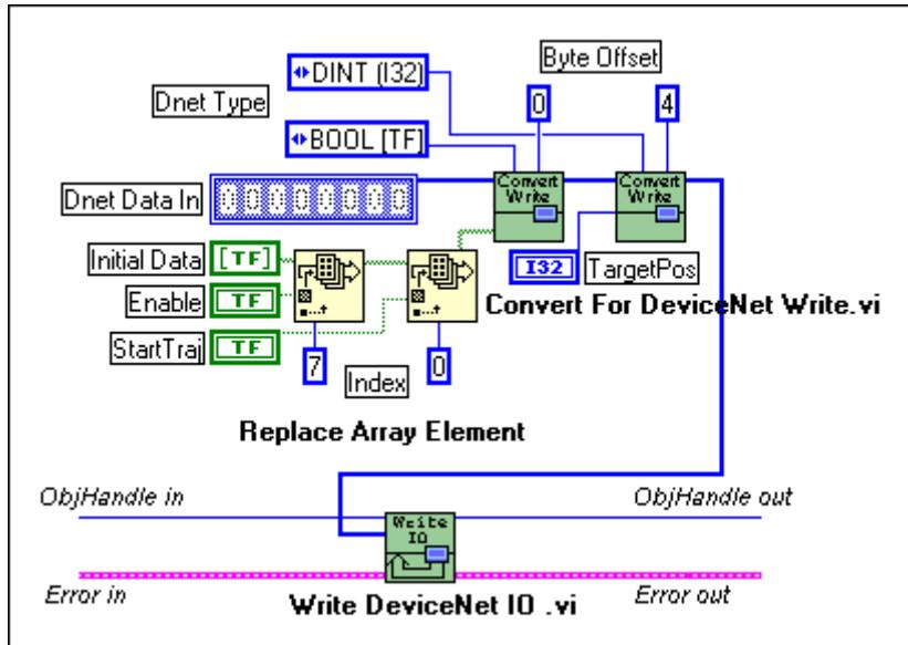
2. Set an attribute Foo using the ncSetDnetAttribute function. The attribute Foo is contained in an object with class ID D5 hex, instance ID 1, attribute ID 5, and its DeviceNet data type is LREAL. Use ncConvertForDnetWrite to convert the appropriate LabVIEW data type for Foo.
