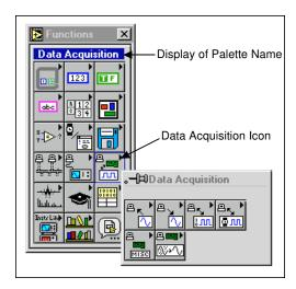
Figure 3-1. Accessing the Data Acquisition Palette
