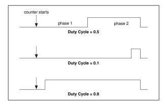
Figure 24-1. Pulse Duty Cycles
