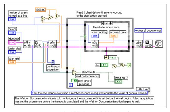
Figure 7-11. Continuous Acq&Chart (Async Occurrence) VI
