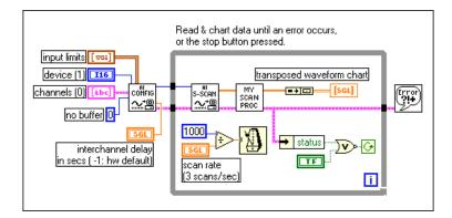
**Figure 6-6.** The Cont Acq&Chart (Immediate) VI Block Diagram
