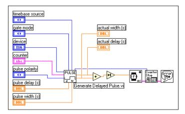
Figure 24-6. Diagram of Delayed Pulse-Easy (DAQ-STC) VI
