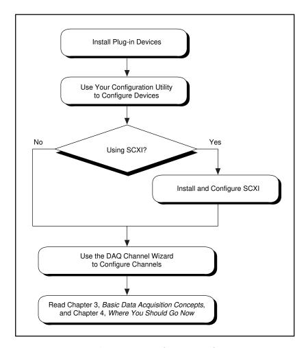
Figure 2-1. Installing and Configuring DAQ Devices
