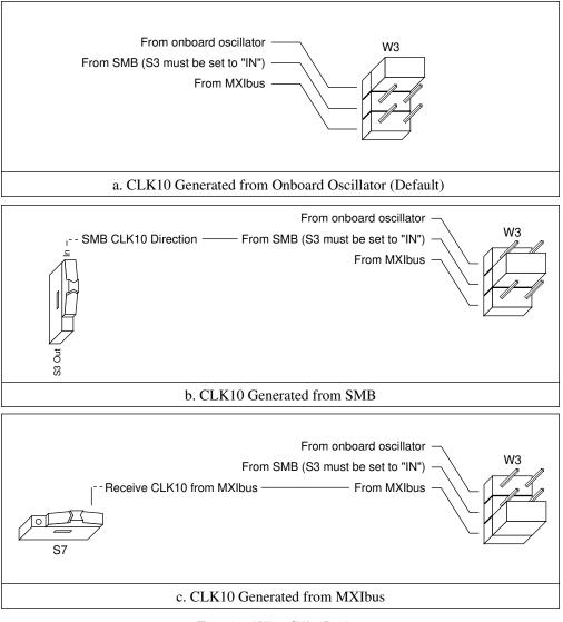
Figure 3-5. VXIbus CLK10 Routing
