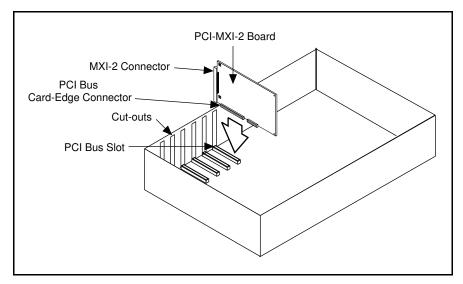
Figure 2-2 shows how to install the PCI-MXI-2.
