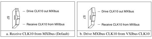
Figure 3-7. Receiving or Driving MXIbus CLK10
