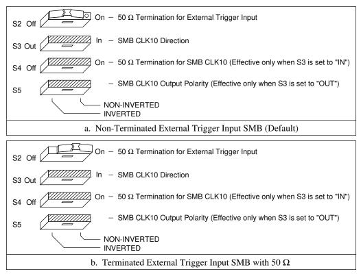
Figure 3-8. SMB Trigger Input Termination
