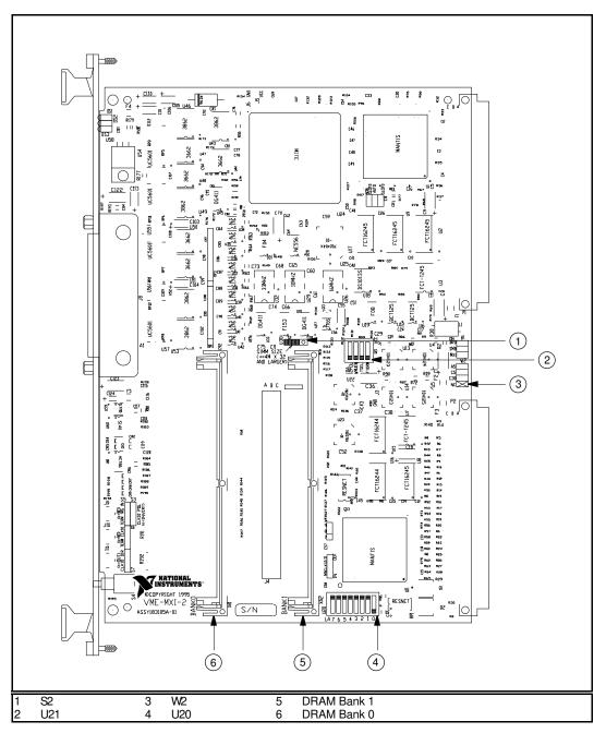
Figure 4-1. VME-MXI-2 Parts Locator Diagram
