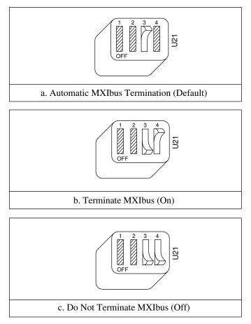
Figure 4-4. MXIbus Termination
