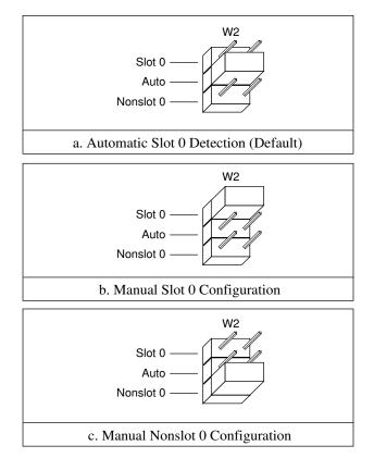
Figure 3-3. VXIbus Slot Configuration
