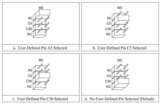
Figure 4-3. VME-MXI-2 Intermodule Signaling Settings
