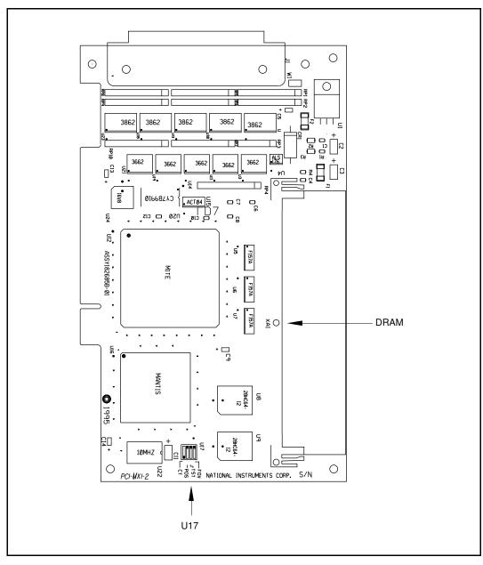
Figure 2-1. PCI-MXI-2 Parts Locator Diagram
