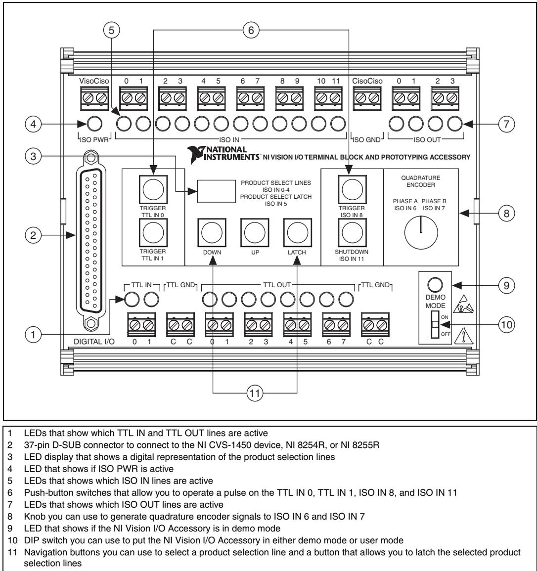
**Figure 1.** NI Vision I/O Accessory Front Panel
