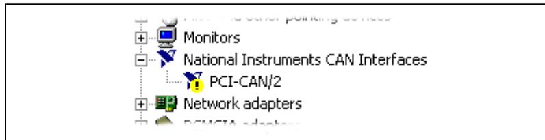
**Figure C-1.** CAN Interface That Is Not Working Properly
