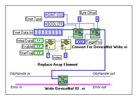
2. Set an attribute Foo using the ncSetDnetAttribute function. The attribute Foo is contained in an object with class ID D5 hex, instance ID 1, attribute ID 5, and its DeviceNet data type is LREAL. Use ncConvertForDnetWrite to convert the appropriate LabVIEW data type for Foo.
