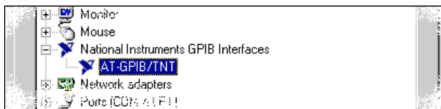
Figure 2-13. GPIB Interface That Is Working Properly
