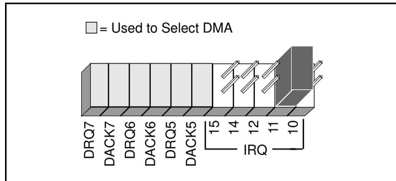
**Figure 2-9.** Interrupt Jumper Setting for IRQ11 (Default Setting)
