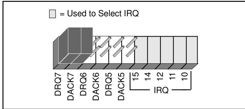
Figure 2-11. DMA Jumper Setting for DMA Channel 7
