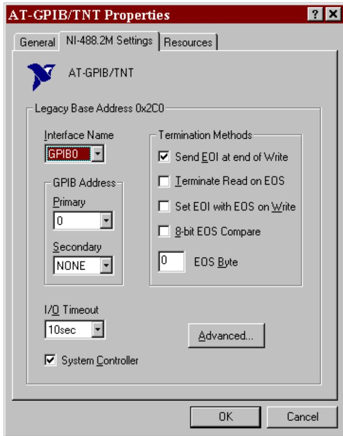
Figure 2-15. NI-488.2M Settings Page for the AT-GPIB/TNT
