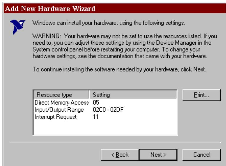
Figure 2-4. AT-GPIB/TNT Resources Assigned Successfully
