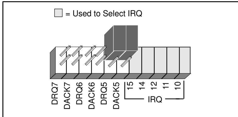
Figure 2-12. DMA Jumper Setting for No DMA Channel
