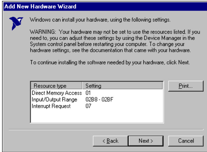
Figure 2-4. AT-GPIB/TNT Resources Assigned Successfully
