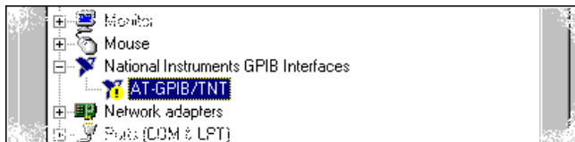
Figure 2-16. GPIB Interface That Is Not Working Properly
