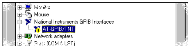
Figure C-1. GPIB Interface That Is Not Working Properly
