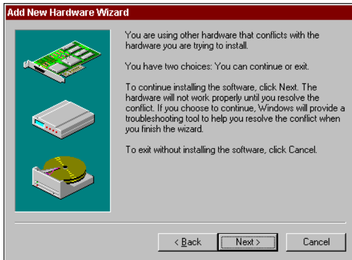
Figure 2-5. AT-GPIB/TNT Resources Not Assigned Successfully
