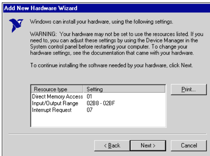
Figure 2-2. GPIB-PCII/IIA Resources Assigned Successfully
