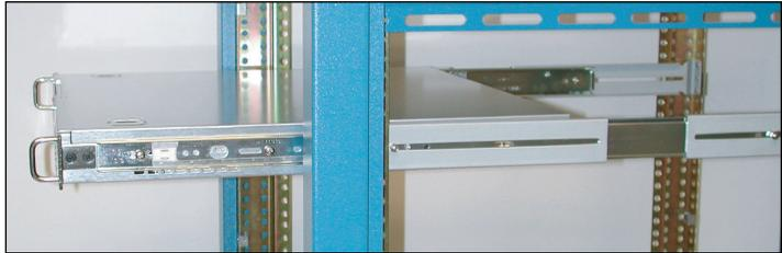
6. Press the locking tabs on both sides of the NI 8350 and slide the NI 8350 fully into the rack.
