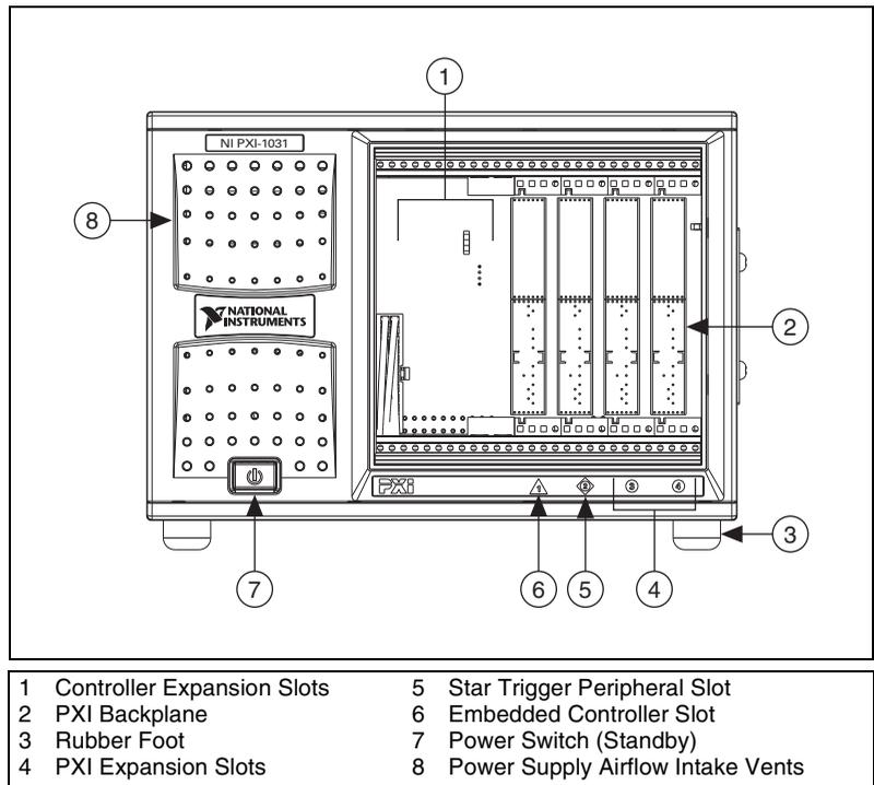
**Figure 1-1.** Front View of the PXI-1031 Chassis
