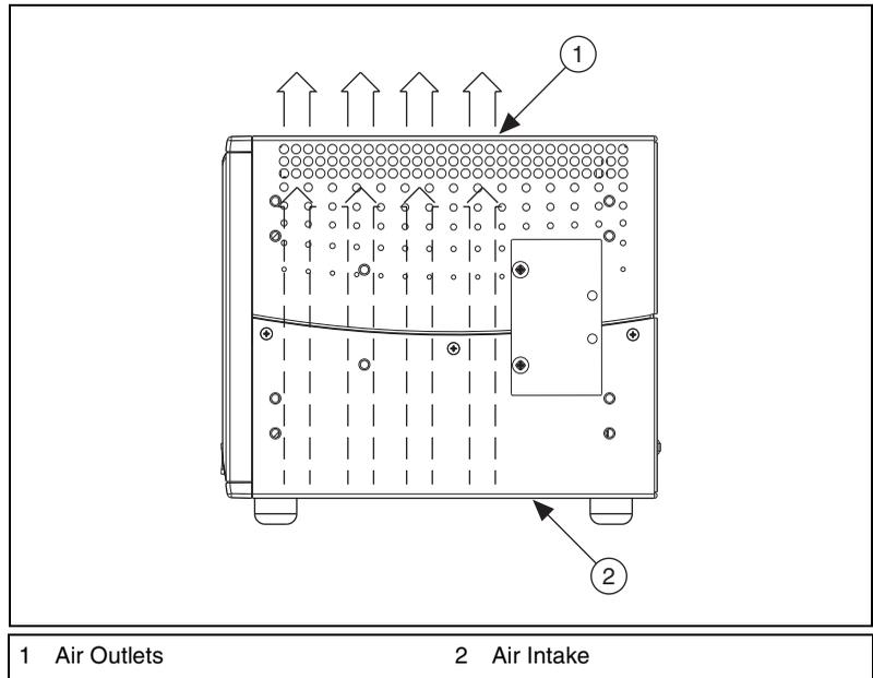
**Figure 2-1.** PXI-1031/PXI-1031DC Module Cooling Airflow Side View
