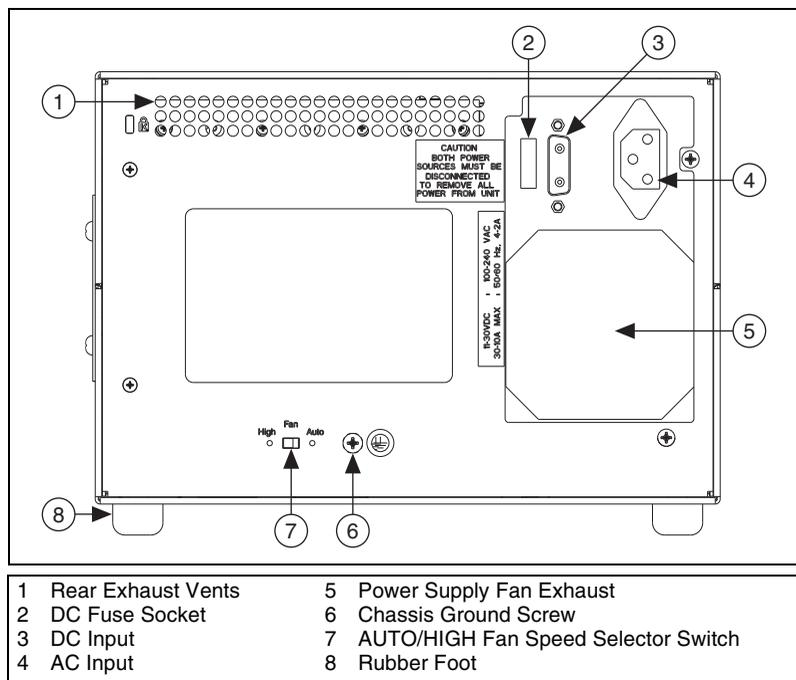
Figure 1-3. Rear View of the PXI-1031DC Chassis
