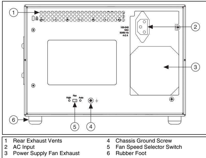
Figure 1-2. Rear View of the PXI-1031 Chassis
