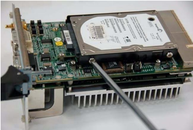
3. Gently pull out the SATA hard drive. Be careful not to bend or break the SATA Board-to-Board connector.
