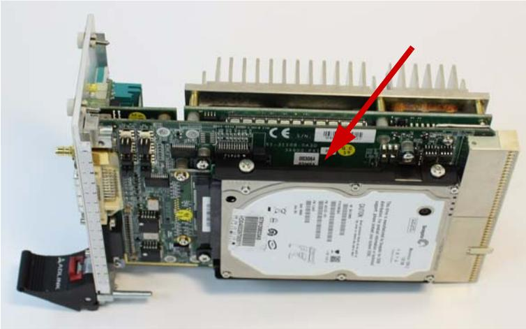
2. Insert the CF card and press down to make sure it is firmly attached in its socket.
