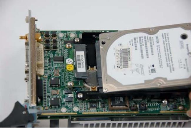
4. To replace the HD with your choice of solid state hard drive or other compatible SATA hard drive, follow the revers steps, and re-install the PXI-3950 to your PXI system.
