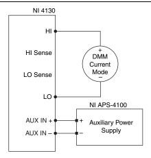
Table 7 lists the test points you must request from the NI 4130 in DC Voltage mode and measure with the DMM to complete verification. For each iteration, set the current limit of the NI 4130 to the value in the *Output* column of Table 7.
