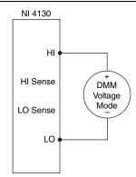
Figure 13. Voltage Adjustment Connection Diagram
