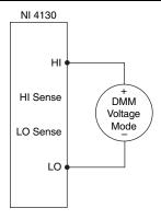
Table 5 lists the voltage test points for each channel that you must request from the NI 4130 and measure with the DMM to complete verification. Take voltage measurements using the DMM at each test point, and compare the result to the programmed voltage value from the *Output* column of Table 5 to calculate the output error. Compare the output error to the *Test Limit* for the iteration of channel *x* in Table 5. If the output error is outside the test limit, adjust the NI 4130.
