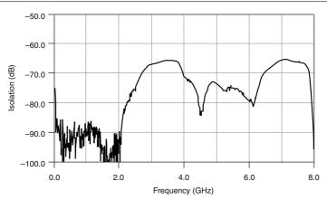
Figure 3. Measured Input to Output Leakage
