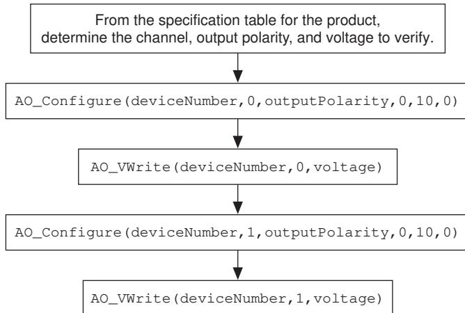
**Figure 2.** Analog Output Verification
