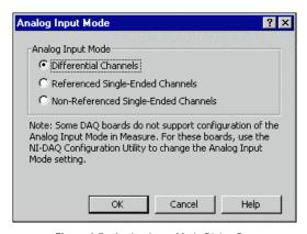
Figure 4-5. Analog Input Mode Dialog Box
