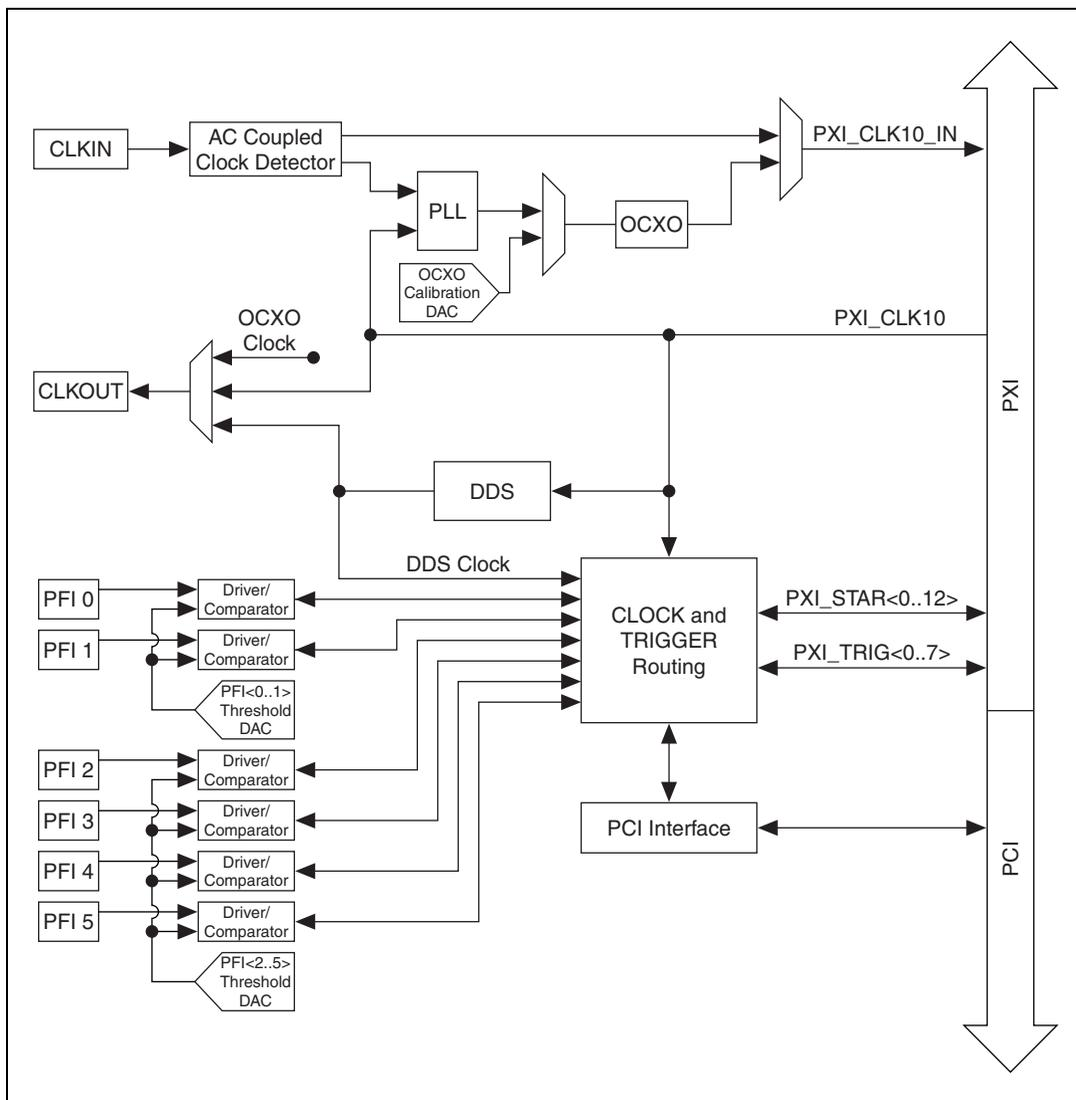
**Figure 3-1.** Functional Overview of the NI PXI-6653
