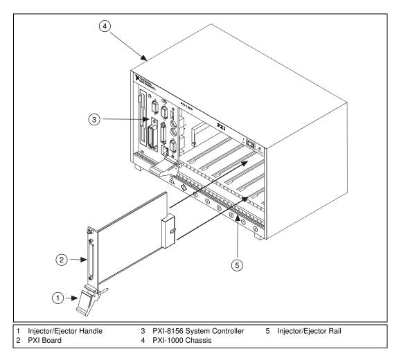
Figure 2-1. PXI Mainframe and Controller
