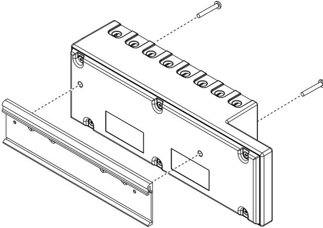
1. Align the NI 9154 and the DIN rail clip.
