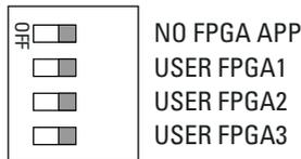
All of the DIP switches are in the OFF position when the chassis is shipped from National Instruments.
