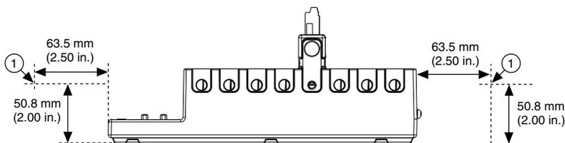
1. Location for measuring the ambient temperature
