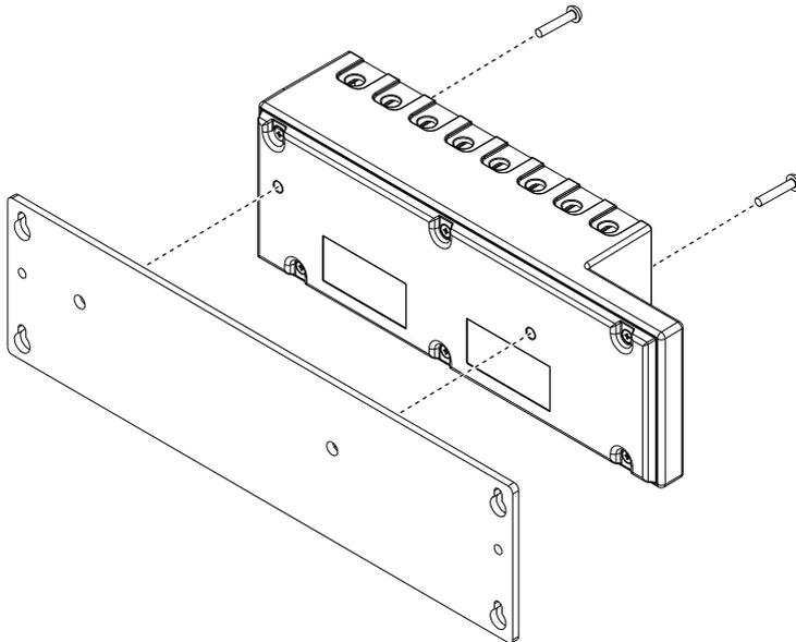
1. Align the NI 9154 and the panel mounting plate.
