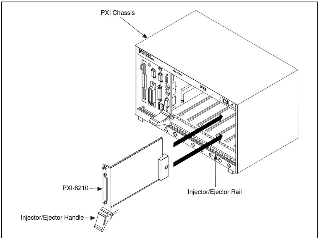
**Figure 1.** Installing the PXI-8210 into a PXI/CompactPCI Chassis
