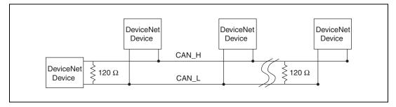
Figure B-7. Termination Resistor Placement
