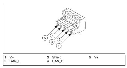
Figure B-1. Pinout for 5-Pin Combicon-Style Pluggable Screw Terminal
