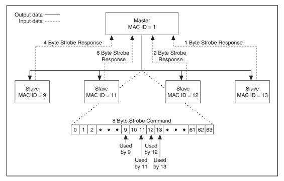
Figure A-4. Strobed I/O Example
