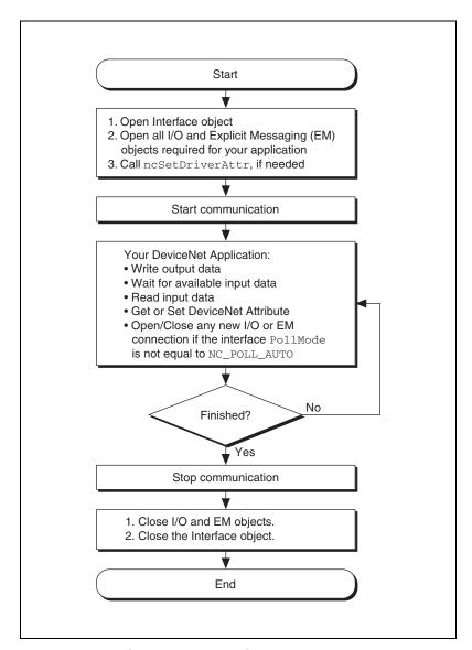
Figure 3-1. General Programming Steps for an NI-DNET Application
