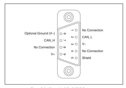
Figure B-3. Pinout for 9-Pin D-SUB Connector
