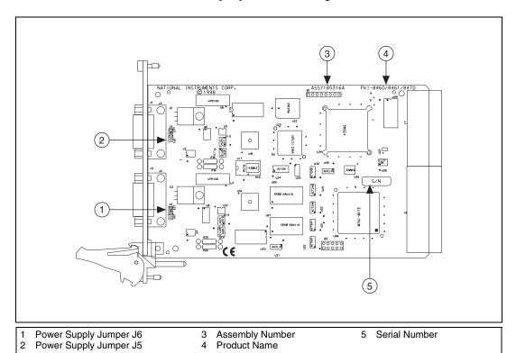
Figure B-6. PXI-8461 Parts Locator Diagram
