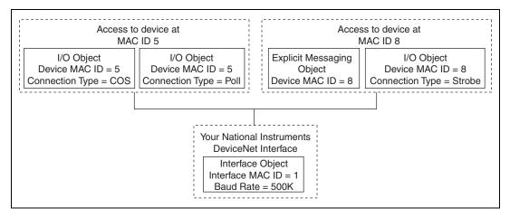
Figure 1-2. NI-DNET Objects for a Network of Three Devices
