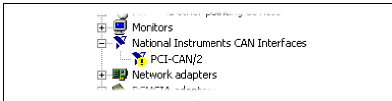
Figure C-1. CAN Interface That Is Not Working Properly
