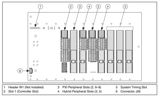
Figure 8. PXI, W1, and J26 Connectors
