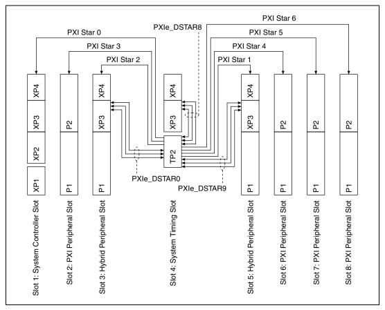
Figure 2. PXIe\_DSTAR and PXI Star Connectivity Diagram
