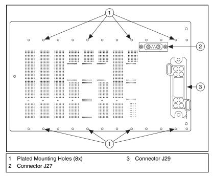
Figure 9. Backplane Power and CLK10 Connectors
