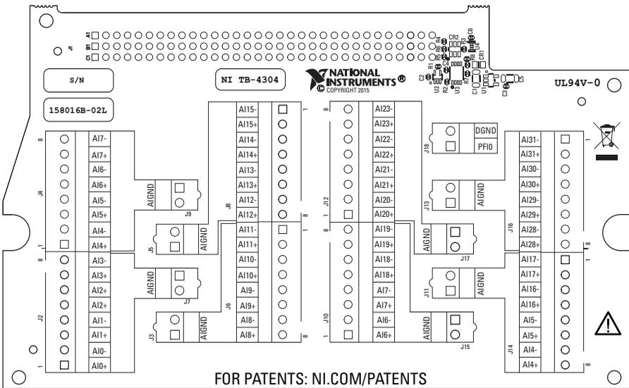
Each channel consists of two terminal connections specific to that channel as shown in Table 2. You can verify or adjust the accuracy for any or all channels depending on the desired test coverage. Refer to Figure 2 and only connect the input channels required for verification or adjustment in parallel.
