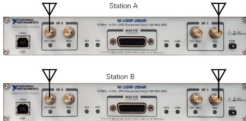
Figure 4 Antenna Connection for USRP RIO Devices
