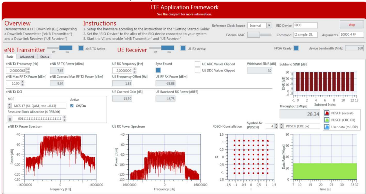
Figure 7 Front Panel of LTE Host DL.gvi / Basic Tab When Running Successfully
