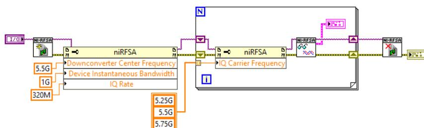
The following figure shows three acquisitions with only digital frequency shift reconfigurations.
