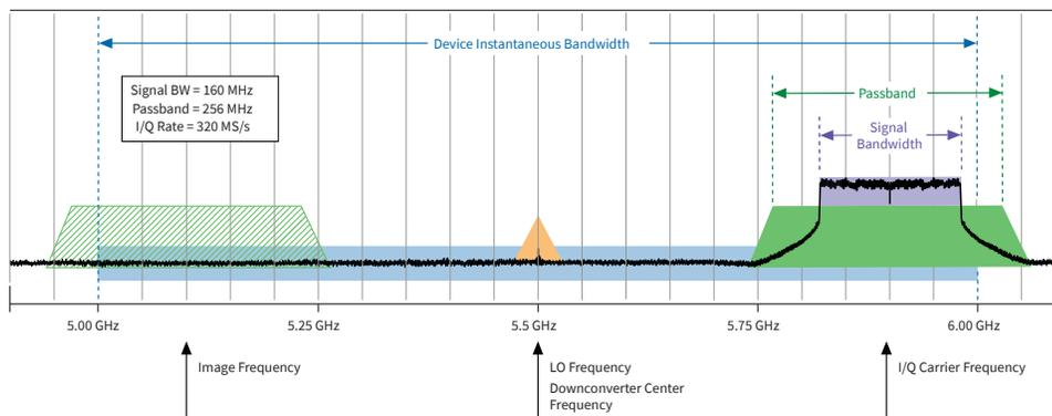
Note that setting the signal bandwidth does not necessarily avoid hardware reconfigurations during in-band retuning, but the settings stay relative to the I/Q carrier frequency, so it may be easier to manage in your application. The following example shows three acquisitions with the same I/Q rate, signal bandwidth, and
