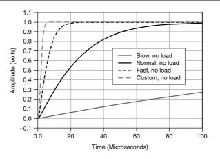
Figure 7. 1 mA Range, No Load Step Response, Nominal
