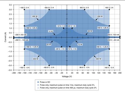
DC sourcing power is limited to 20 W, regardless of output voltage.<sup>4</sup>
