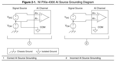
The COM terminal for each channel must be connected to the reference ground of the AI source. Failure to connect COM results in inaccurate measurements. You can connect the COM terminal directly to the negative terminal of the source as shown in Figure 2-1 or to an isolated ground of the source as long as the working voltage specification of the NI PXIe-4300 is not violated.
