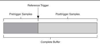
Figure 2-8. Reference Trigger Final Buffer
