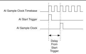
Figure 2-6. Al Sample Clock and Al Start Trigger
