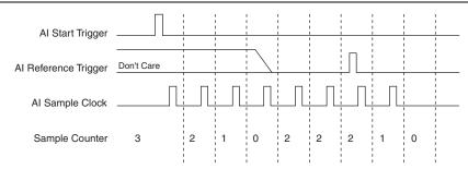
Figure 2-5. Typical Pretriggered DAQ Sequence
