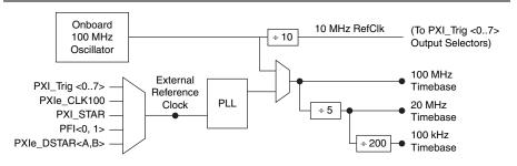
**Caution** Do not disconnect an external reference clock once the modules have been synchronized or are used by a task. Doing so may cause NI-DAQmx to return an error. Make sure that all tasks using a reference clock are stopped before disconnecting it.
