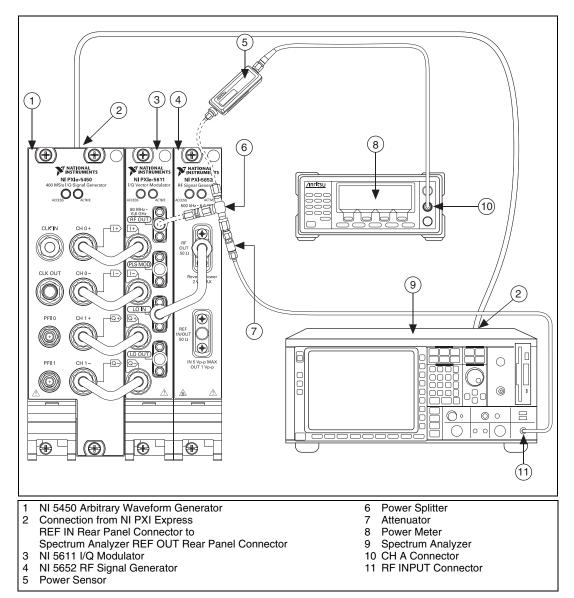
Figure 3. Connecting Hardware to Verify RF Path Gain
