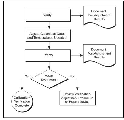
Figure 1 shows the programming flow for a complete calibration.
