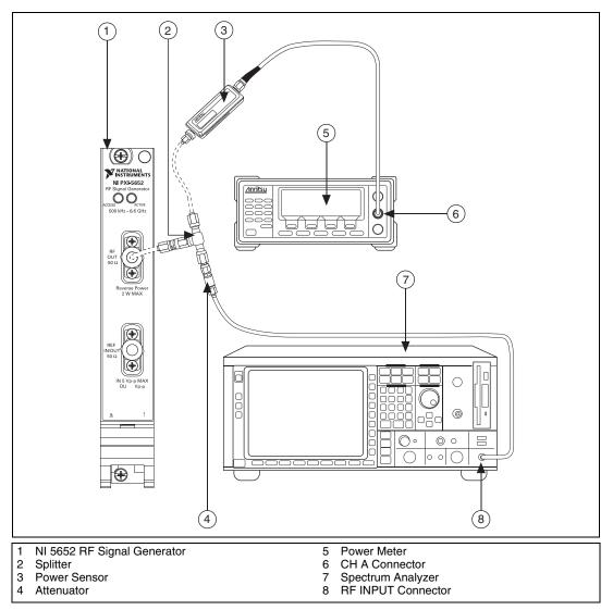
Figure 2. Power Splitter Characterization Setup
