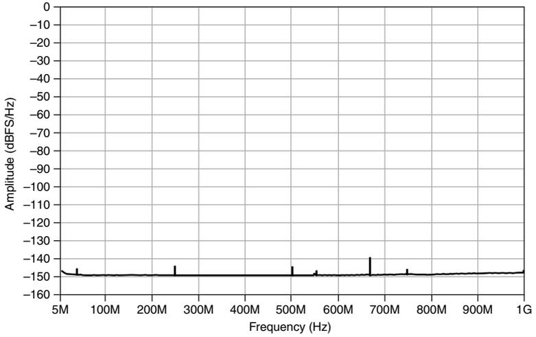
**Figure 6.** Measured Input Terminated Noise Density<sup>16</sup>, Dither On, Digitizer Mode
