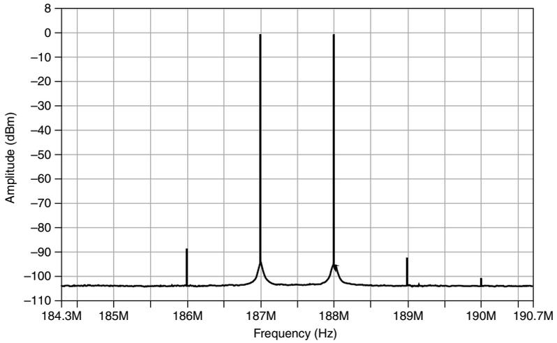
**Figure 10.** Measured Two-Tone Spectrum, 730 MHz Center Frequency, DDC Mode<sup>27</sup>
