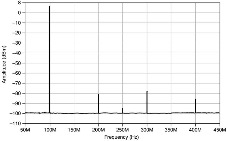
**Figure 8. Measured Single-Tone Spectrum, 800 MHz Instantaneous Bandwidth, DDC Mode<sup>25</sup>**
