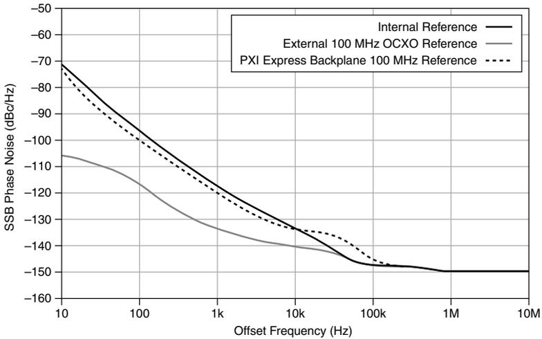
**Figure 2. Measured SSB Phase Noise<sup>9</sup> of Internal Reference, Multiple Carrier Frequencies<sup>10</sup>**
