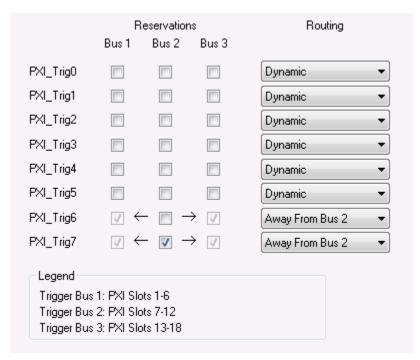
Figure 1: Example Trigger Routing in MAX
