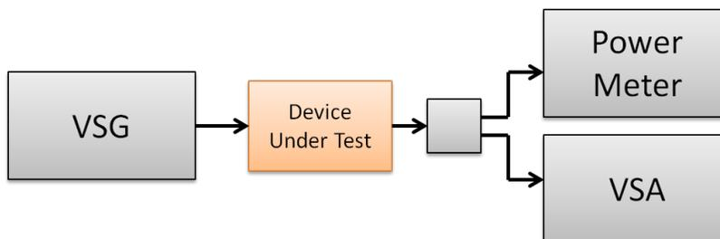
Figure 1. Traditional PA Test Setup
