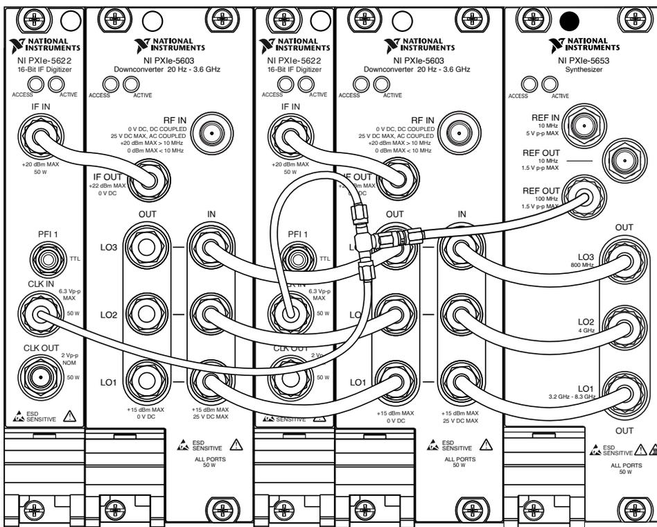
The following figure shows an interconnected PXIe-5665 (14 GHz) using two RF signal downconverters and two IF digitizers.
