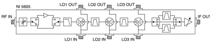
The PXIe-5605 RF front end includes a mechanical step attenuator, which is variable up to 75 dB in 5 dB steps. When the PXIe-5605 is operating in the low band signal path, the solid-state attenuator provides an additional 31 dB of attenuation, variable in 1 dB steps. The RF input is AC-coupled by default, but you can also configure the input to be DC-coupled using NI-RFSA.
