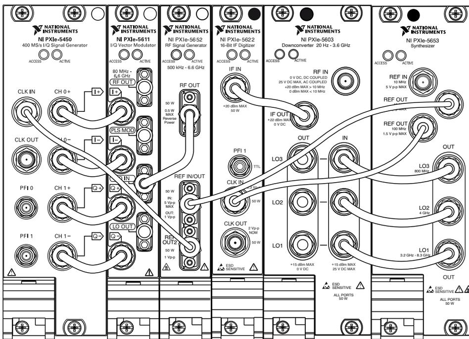
The following figure shows an interconnected PXIe-5665 (14 GHz) and PXIe-5673E using an internal clock.
