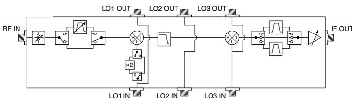
The only available attenuation in this frequency band is the mechanical step attenuator, which provides 75 dB of attenuation, variable in 5 dB steps. An optional preselector assists in filtering unwanted frequency components from the RF input before the signal reaches the first mixer.
