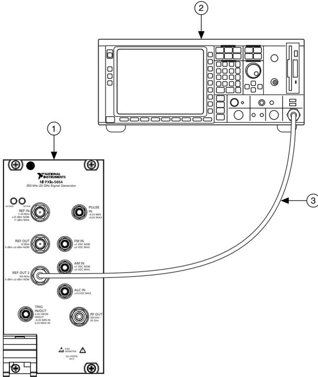
1. PXIe-5654 RF Analog Signal Generator
