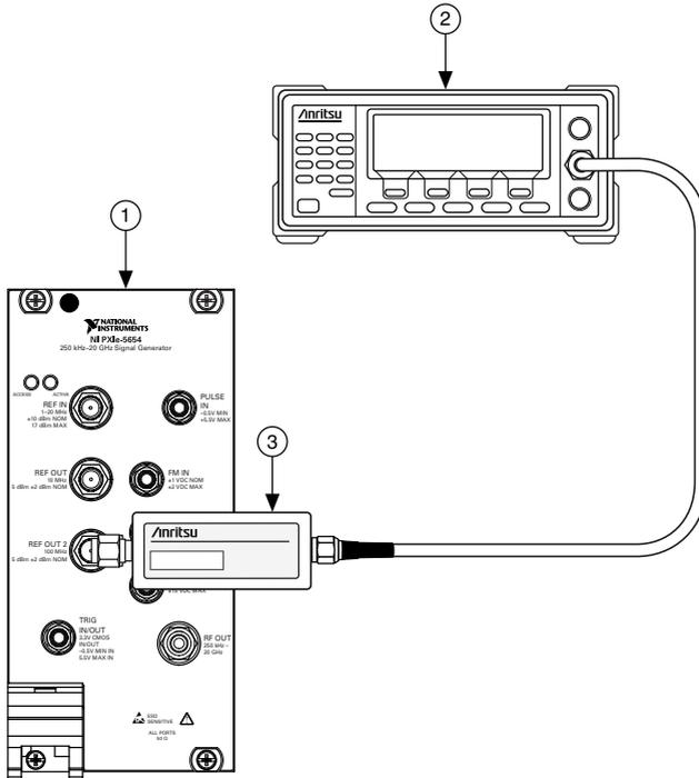
1. PXIe-5654 RF Analog Signal Generator
