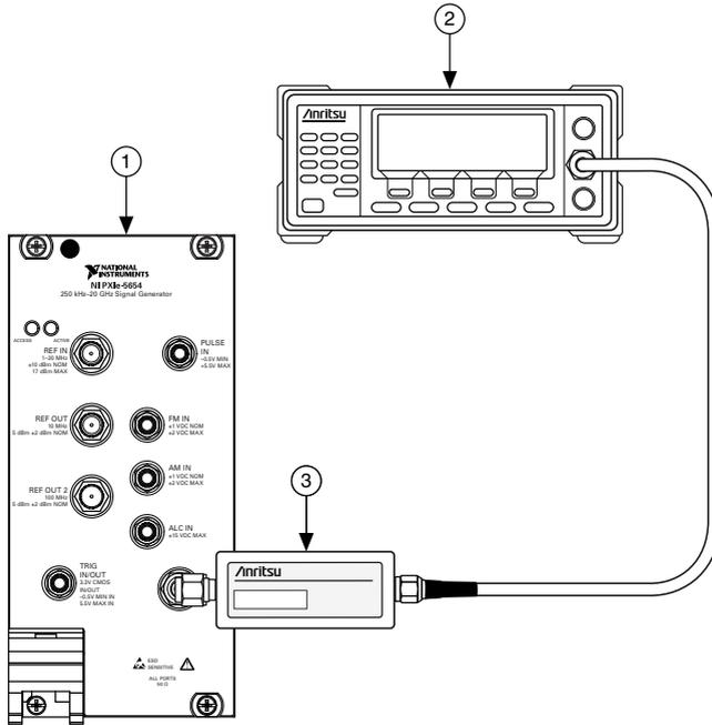
1. PXIe-5654 RF Analog Signal Generator
