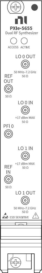
Figure 2. PXIe-5655 with MMPX Front Panel
