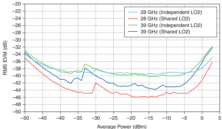
Figure 39. Direct TRX to Switched RF 5G NR 1 CC x 100 MHz RMS EVM versus Average Power, Measured 33,34
