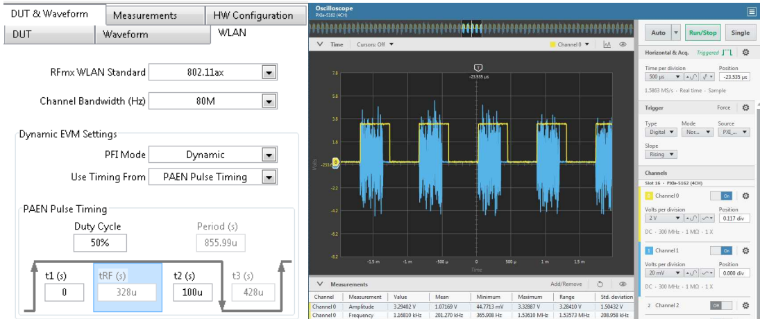
Figure 11: Scope Trace of RF and Enable Pulse in Dynamic/PAEN Pulse Timing Mode
