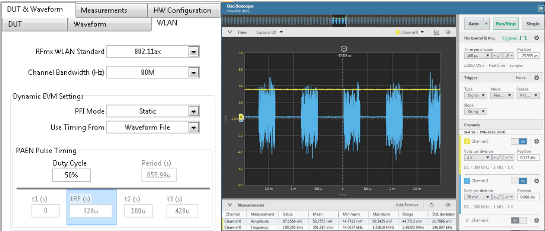
Figure 9: Scope Trace of RF and Enable Pulse in Static/Waveform File Mode
